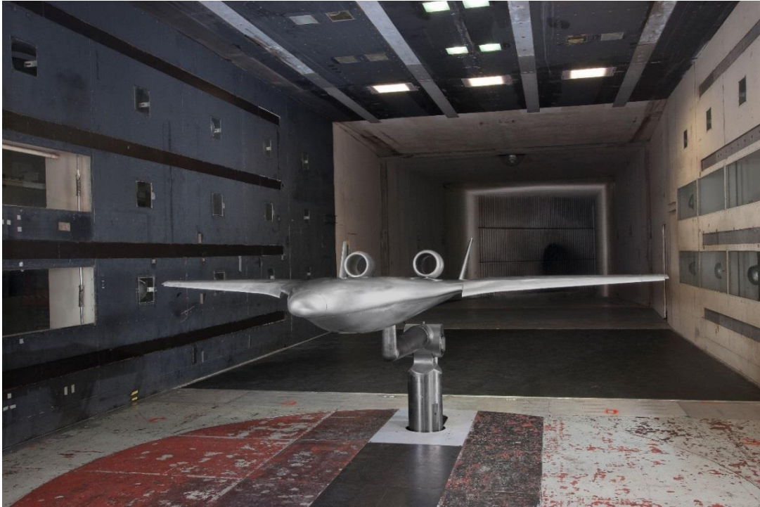
Figure B-5 Aerodynamic Test of the HWB in the 14x22' Subsonic Wind Tunnel (32)
