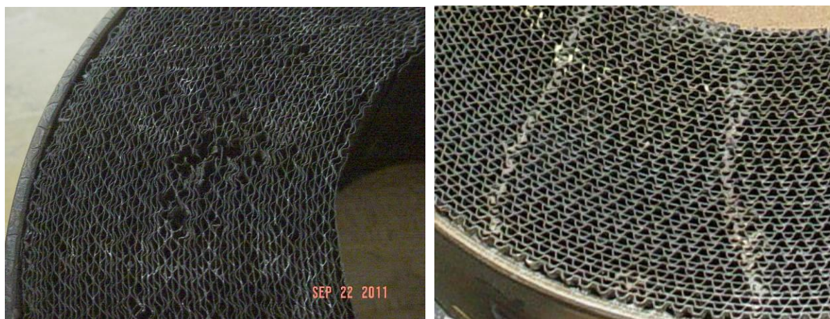
Figure -2 The Effect of Flame Impingement on a Flow Conditioner.
