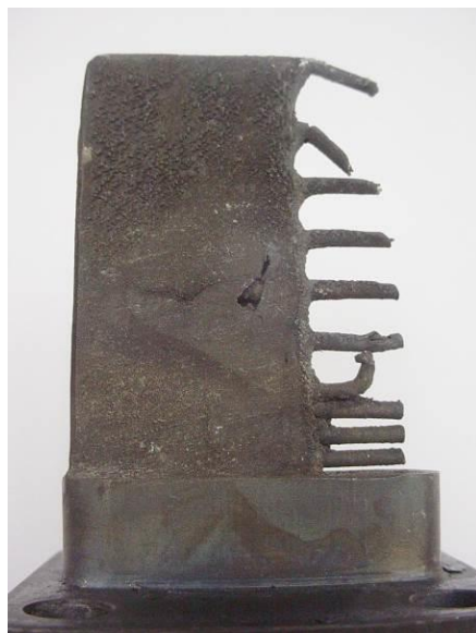
Figure 3 The Effect of Flame Impingement on a Temperature Rake.
