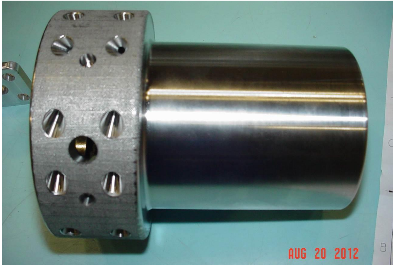
Figure 18 A Finished CoCr Combustor Liner
