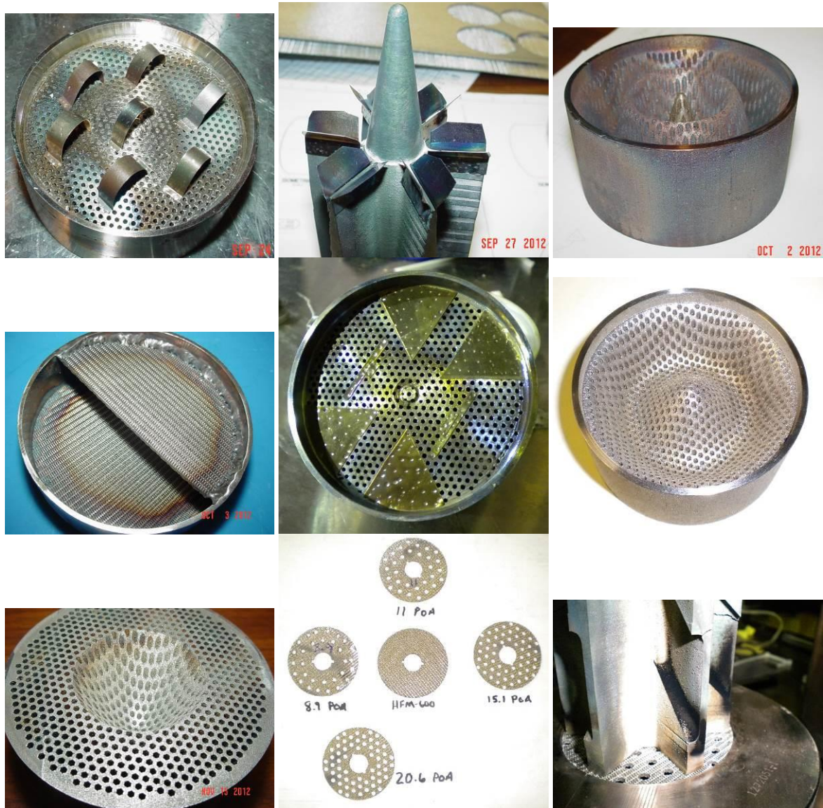
Figure 34 Some of the Combustor Change Variations tried to eliminate the Combustor Instability
